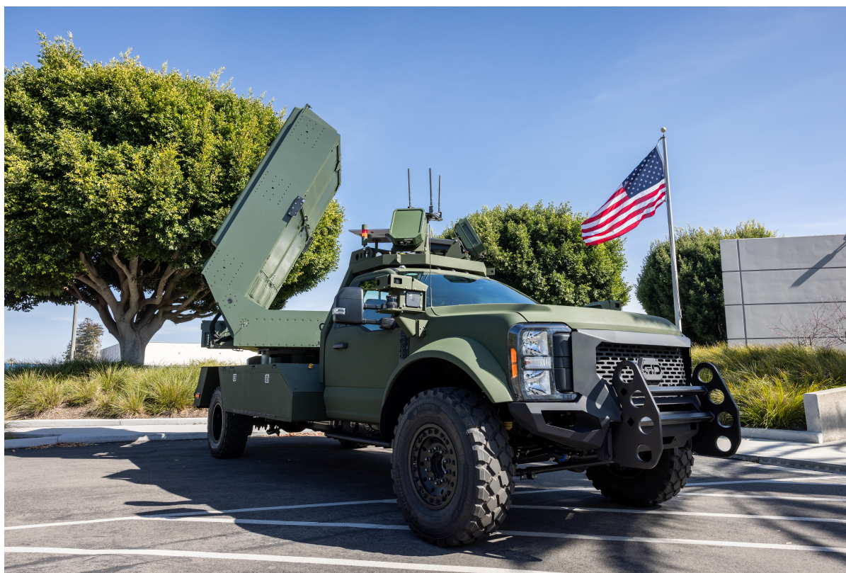
Leonidas Autonomous Ground Vehicle (AGV) combines Epirus' Leonidas high-power microwave platform, the Kodiak Driver autonomous system and General Dynamics Land Systems' system integration expertise to deliver a mobile, autonomous counter-UAS capability
