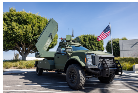
Leonidas Autonomous Ground Vehicle (AGV) combines Epirus' Leonidas high-power microwave platform, the Kodiak Driver autonomous system and General Dynamics Land Systems' system integration expertise to deliver a mobile, autonomous counter-UAS capability
